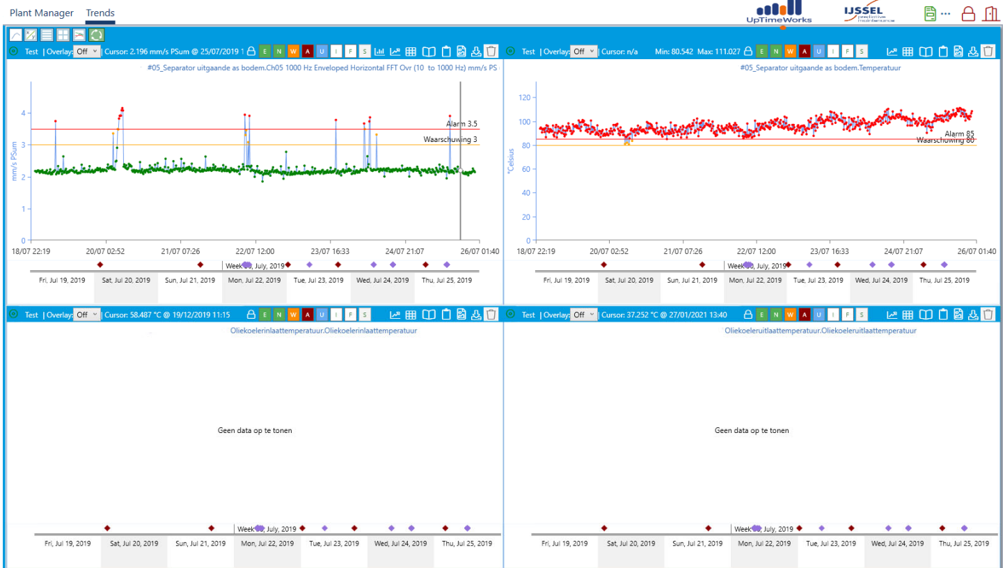
Figure 3: Trend data for the Bottom Output Shaft Separator Module without IJssel's Oil Cooling & Filtration Unit. Clockwise from upper left: Vibration measurements (FFT PEAK; mm/s) shows multiple peaks above alarm values (3-3.5 mm/s); Temperature graph shows a continuous level above alarm values (80-85°C); No data; No data. [Source: UpTimeWorks.com]
