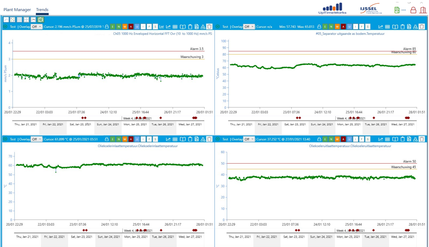
Figure 4: Trend data for the Bottom Output Shaft Separator Module with IJssel's Oil Cooling & Filtration Unit installed. Clockwise from upper left: Vibration measurements (FFT PEAK; mm/s) shows a flared level of peaking below alarm values (3-3.5 mm/s); Temperature graph shows a continuous level below alarm values (80-85°C); Oil Cooling & Filtration Unit outlet temperature graph shows a continuous level below alarm values (45-50°C); Oil Cooling & Filtration Unit inlet temperature. [Source: UpTimeWorks.com]
